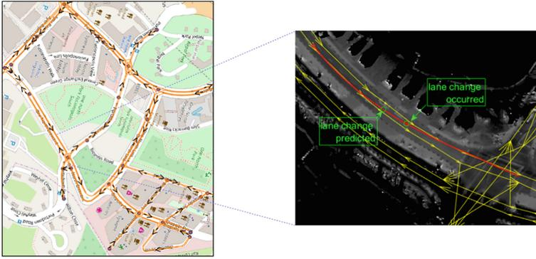
**Fig. 2.** The digital map overlaid with the lane center in yellow (left). A close-up of the digital map illustrating lane-change instance in red (right).
