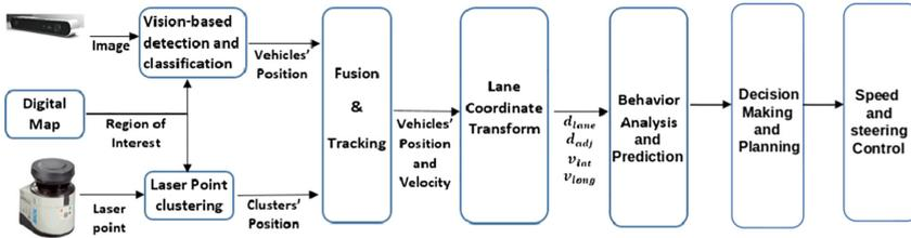
**Fig. 1.** System overview comprising of five modules: perception, sensor fusion and tracking, behavior analysis and prediction, decision making and planning, speed and steering control.
